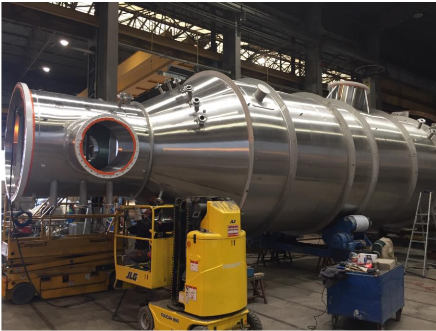
Figure 10: Crystallizer made of UNS N08034 manufactured by ZIEMEX†
